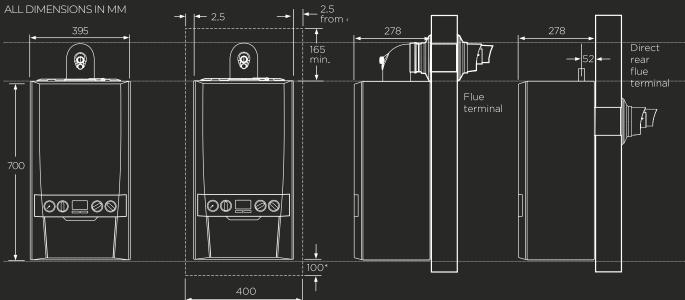
Note: The minimum front clearance when built into a cupboard is 5mm from the cupboard door but 450mm overall clearance with the cupboard door open is required for servicing.
