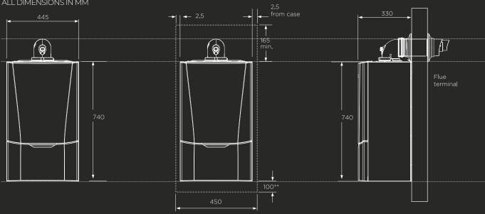
Note: The minimum front clearance when built into a cupboard is 5mm from the cupboard door but 450mm overall clearance with the cupboard door open is required for servicing. \*Bottom clearance after installation can be reduced to 5mm. However, 100mm is required for servicing.
